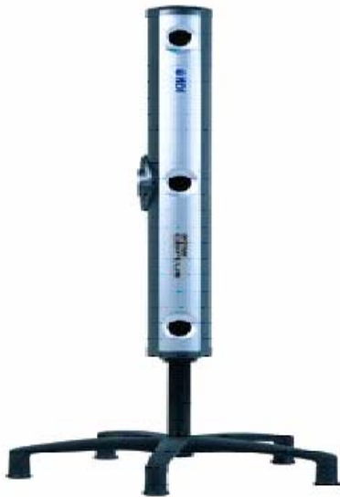
Figure 2.1 The Optotrak® Certus™ 3D motion measurement system (Northern Digital Inc., Waterloo, Ontario, Canada)
