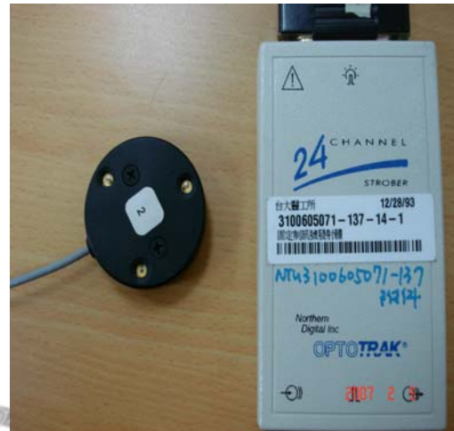
Figure 2.1 The Optotrak® Certus™ 3D motion measurement system (Northern Digital Inc., Waterloo, Ontario, Canada)
