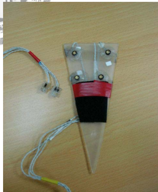
Figure 2.8 The stylus. Use the bottom of cutting-edge of the stylus to point at each specific landmark.
