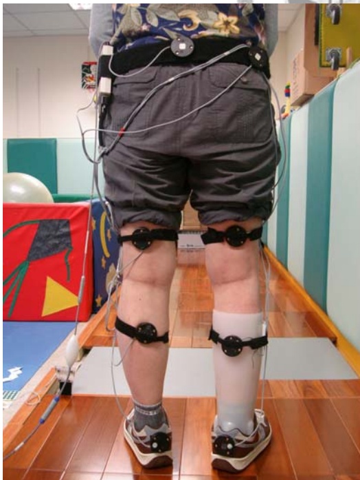
Figure 2.7 Seven rigid body sensors were attached on lower extremities of subjects by Velcro tapes, including bilateral feet, shanks, thighs, and the pelvis.
