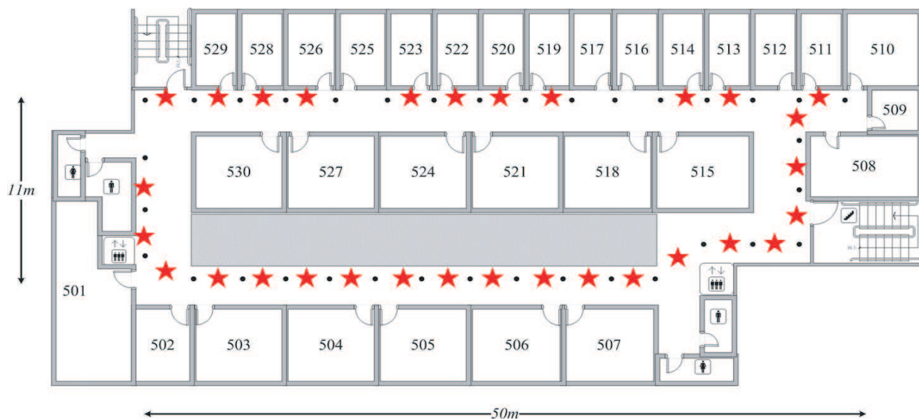
Figure 5.7: The fifth floor plane of the BL building, where we had performed the experiments. The red stars represent the testing locations.
