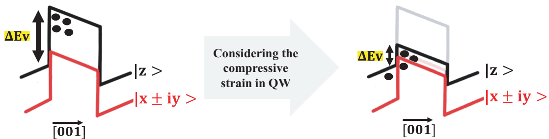
Figure 5.12: The mechanism of strain-induced deformation potential in high Al composition AlGaIn QW region.
