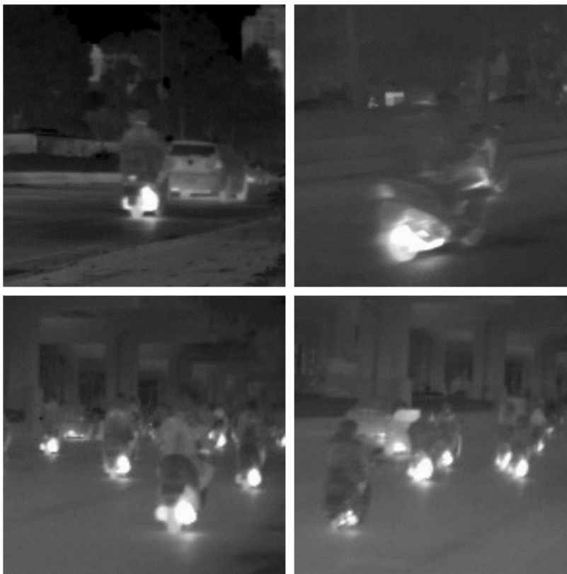
Figure 4- 8 Example of Thermal Image of Motor
