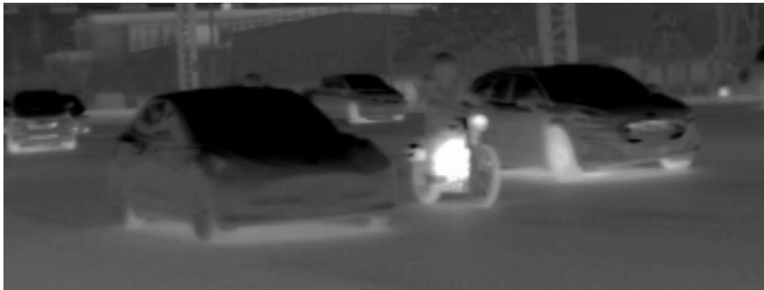
Figure 4- 4 Example of Thermal Image of Cold Car
