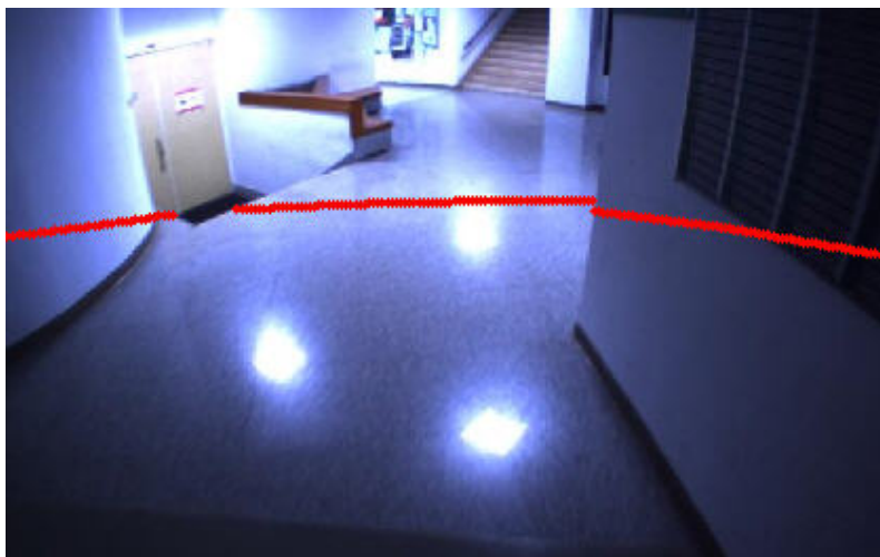
Figure 5.2. Camera-LIDAR calibration results The LIDAR is located below the camera slightly shifted to the left.
