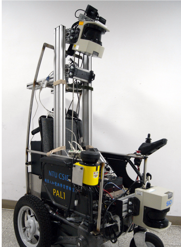
Figure 5.1. Modified PAL1 robot used for experiments. The top SICK LMS was the main sensor used in the experiments. The horizontally oriented LIDAR in the front was used to collect data for performance comparison.
