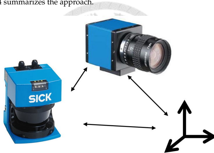
Figure 3.4. Overview of the calibration procedure. First the extrinsic parameters between camera and LIDAR are estimated. Then the camera is located using a checkerboard. Finally the LIDARs pose is found by combining the two previous results.
