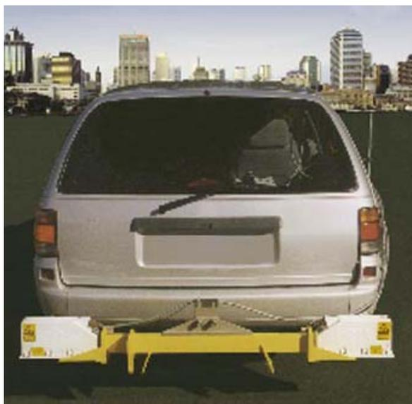
圖2.10 ARRB雷射平坦儀(後保險桿)[7]
