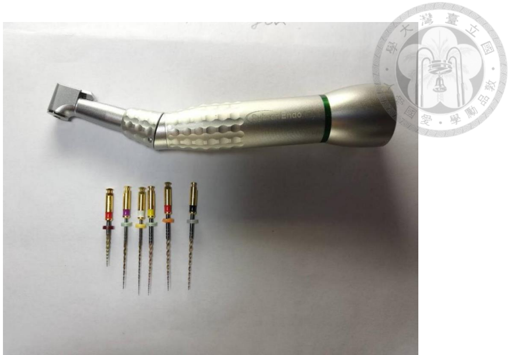
Fig. 16 The rotary machine (Analytic Quintec® ETM, Taiwan, low-speed handpiece 18:1 at 340 rpm) used to collect odontoblastic powder.
