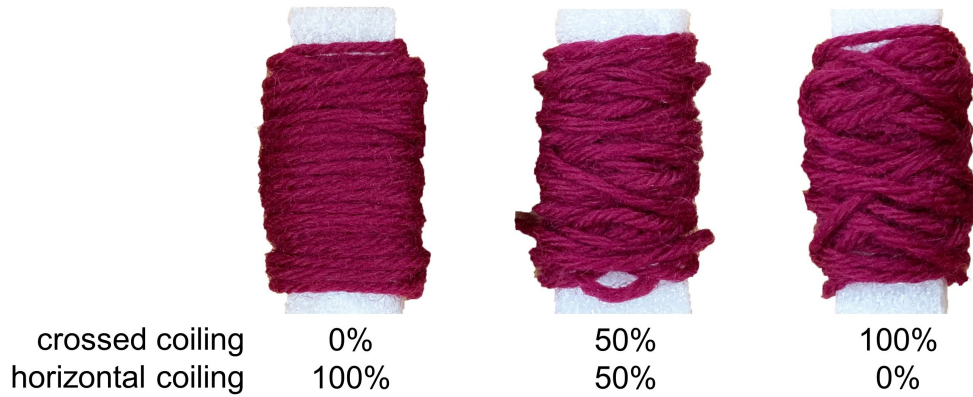
Figure 6.3: The figure demonstrates the cylinder results made with different crossed coiling ratios in the coiling way test.
