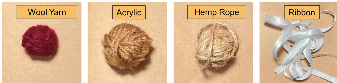
Figure 6.1: The results of the material test by coiling to a ball and then felt it. The wool yarn has the best performance at the compressed and entangled levels. Acrylic and hemp rope' performances are not well enough in compression, and ribbons can not entangle together.
