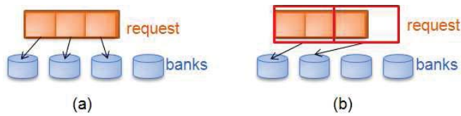
Figure 3.4: Illustration of Different Striping Unit Size. (a) Striping Unit Size = 1 page. (b) Striping Unit Size = 2 pages.
