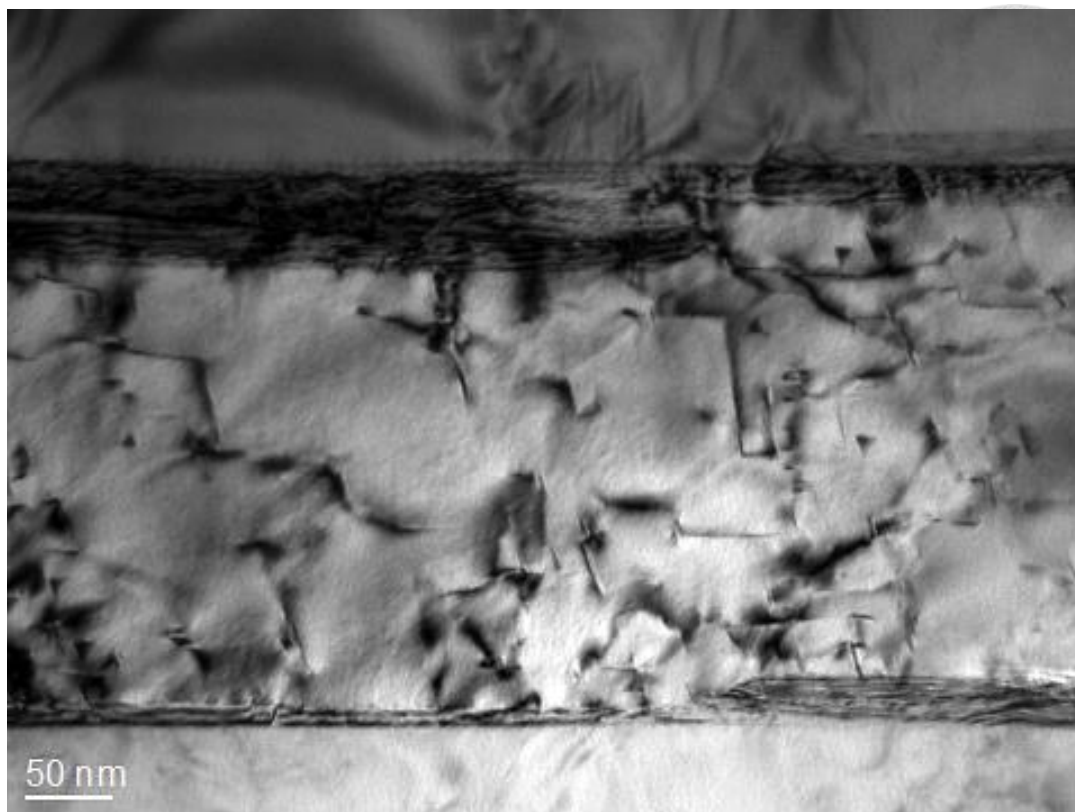
Figure 4-30 TEM image of (\text{CrCoNi})_{94}\text{Al}_3\text{Nb}_3 recrystallization at 900°C for 1 hour before \delta connecting to each other.
