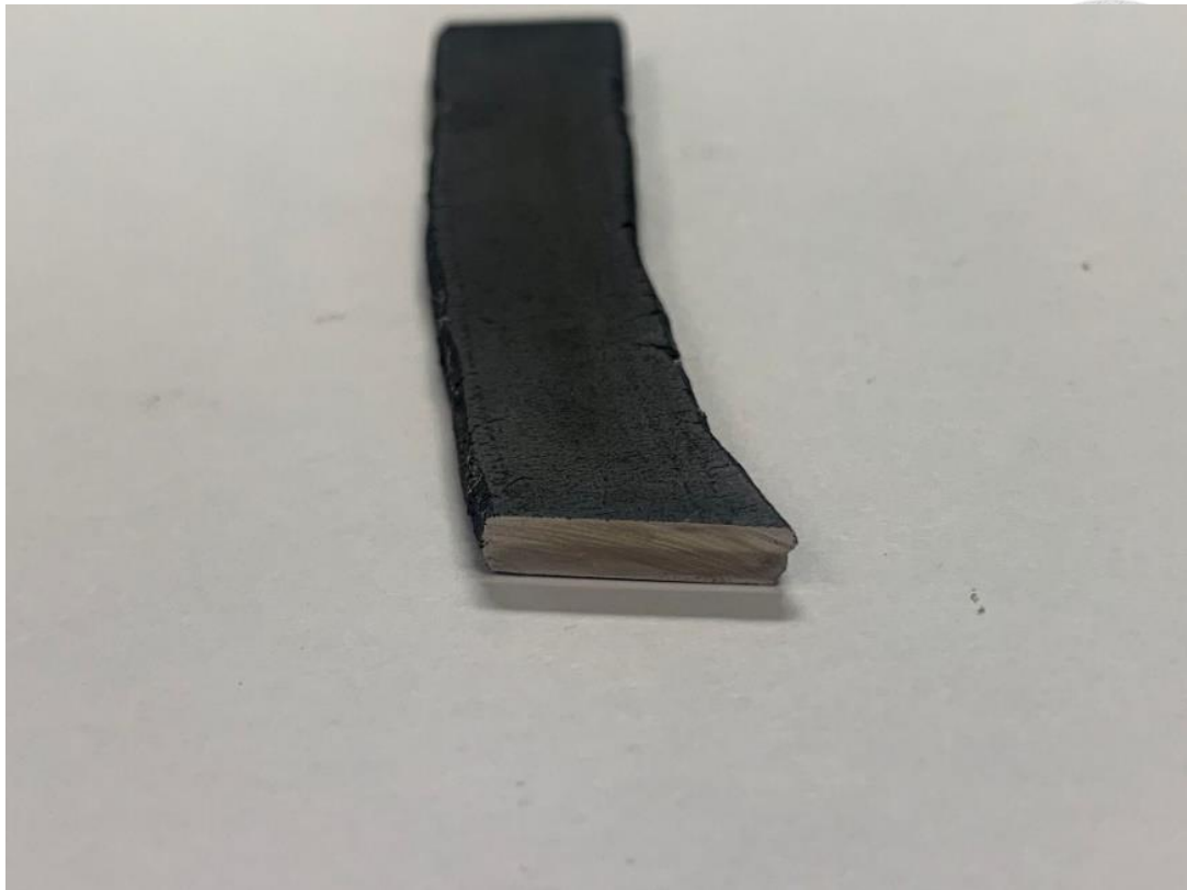
Figure 3-4 Successful hot rolling materials at 1100°C.
