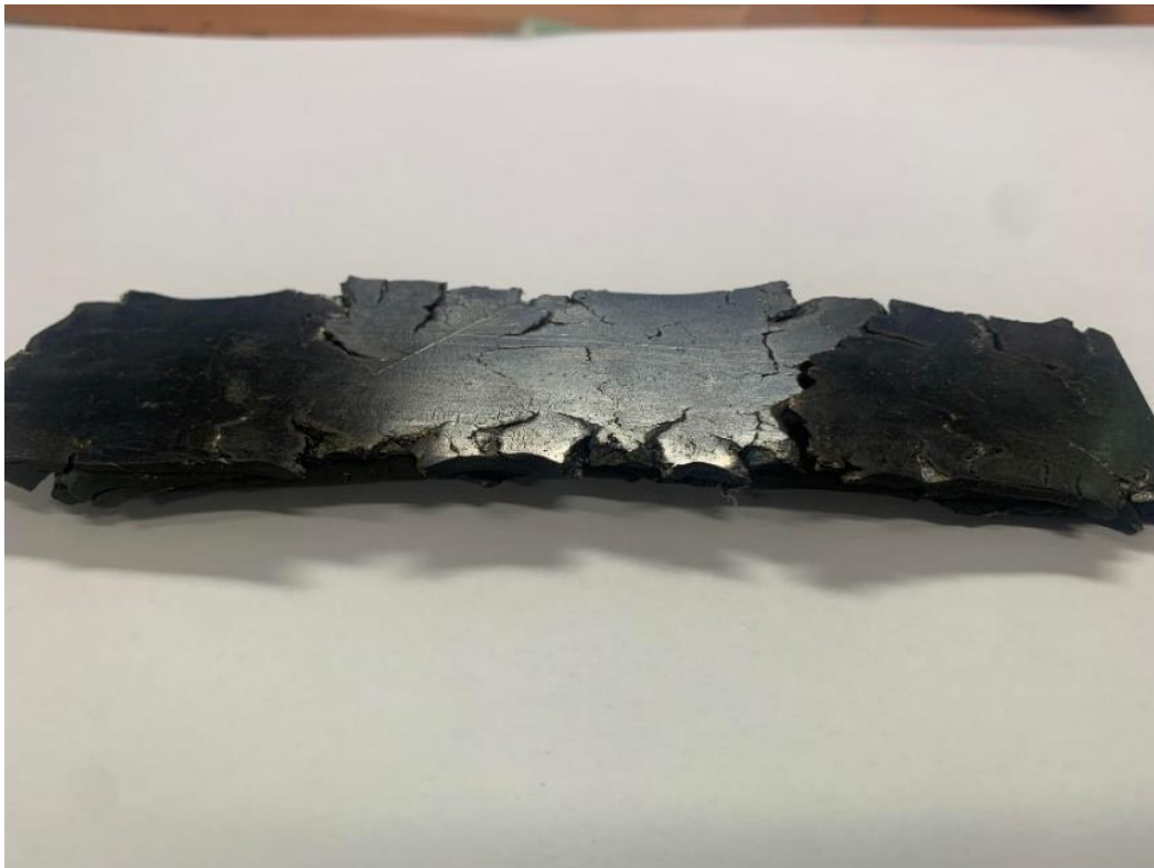
Figure 3-3 Failed hot rolling materials at 1100°C.
