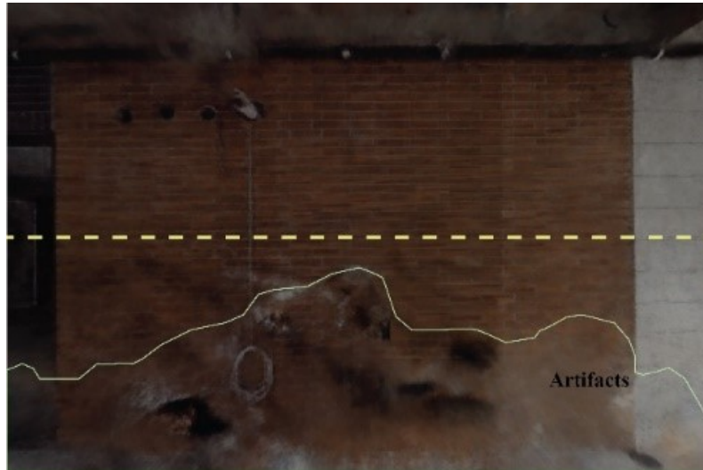
Figure 3.26: Artifacts in the bottom half of the NeRF-generated orthographic image.
