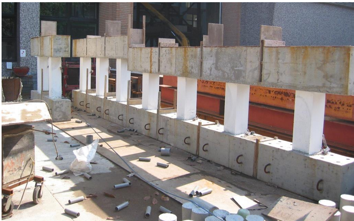
Figure 4-6. Casted shaking table test column specimens (Su 2007)
