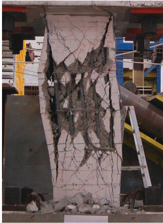
Figure 3-15. Specimen 3NL crack pattern before collapse (5%) (Weng 2007)
