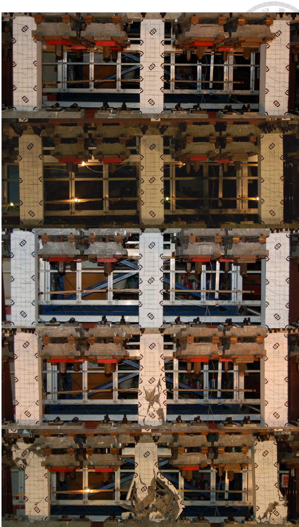
Figure 4-33. T1 Frame crack pattern after each run
