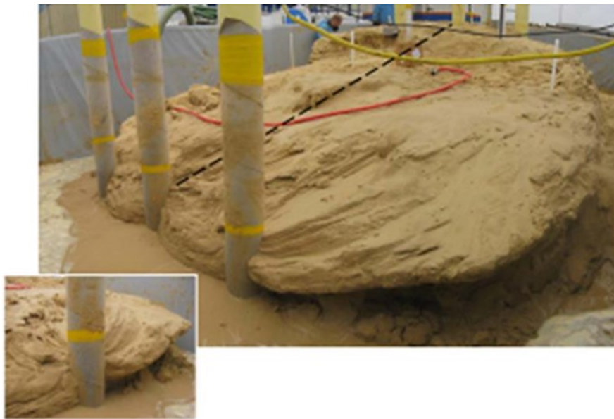
Figure 2.41: 大尺度砂粒固結試驗 (Van Paassen et al., 2010b)
