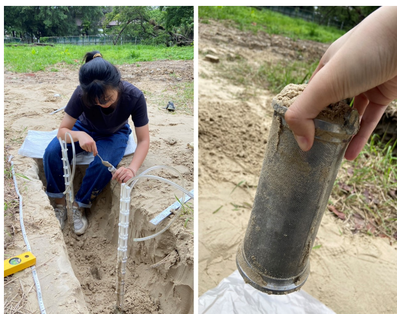
Figure 3.71: 改良試體開挖及取樣
