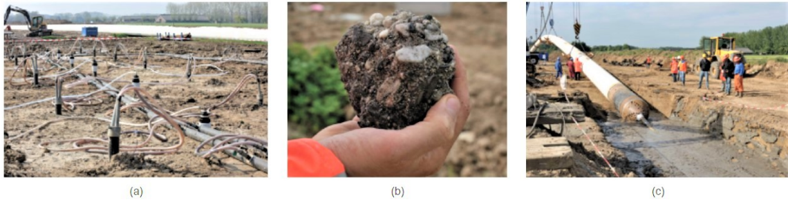
Figure 2.37: 鬆散礫石之固結現地試驗 (Van Paassen, 2011)
