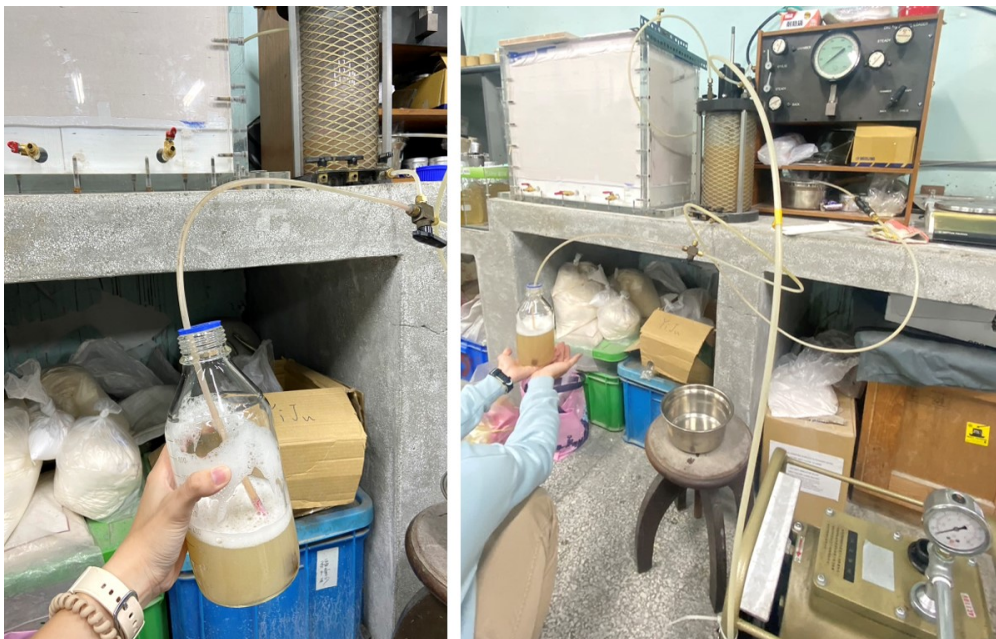
Figure 3.54: 側向加壓滲透之中型砂箱試驗配置
