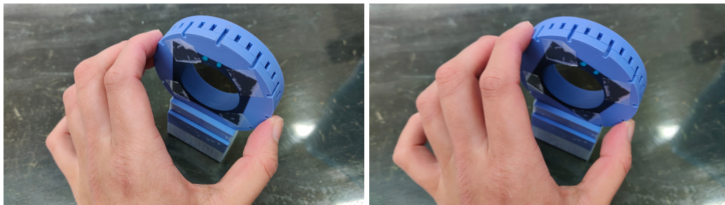
(b) The example figures of how to rotate the analyzer by 20^\circ .
