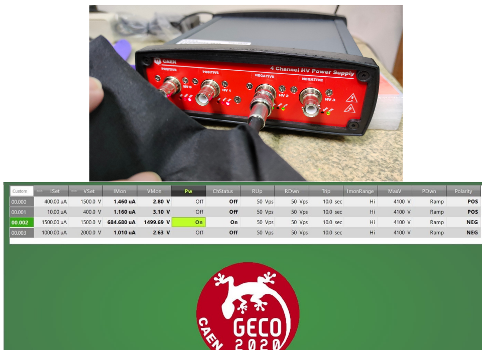
Figure 3.4: The high voltage power supply module DT-5533E from CAEN and its control software GECO.
