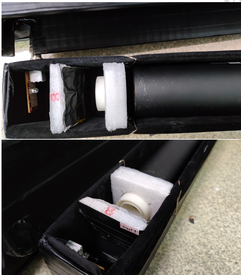
Figure 3.1: The LED calibration setup, from different perspectives.
