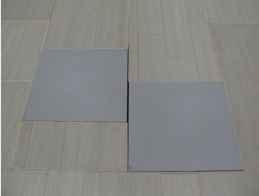
圖 2-2 AMTI® 測力板， Advanced Mechanical Technology Inc, Watertown MA, USA)
