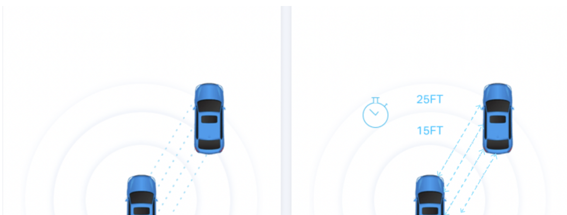
Figure 7: Lidar sensor computes the distance by the reflected pulse [5]
