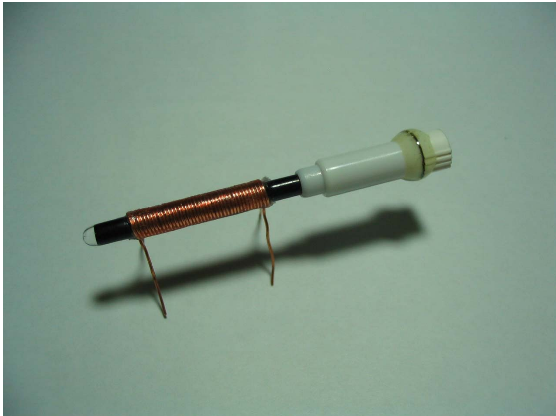
Figure 2.4 The photo of the transformer on a capillary which carries the oil-based \text{Fe}_3\text{O}_4 nanofluid
