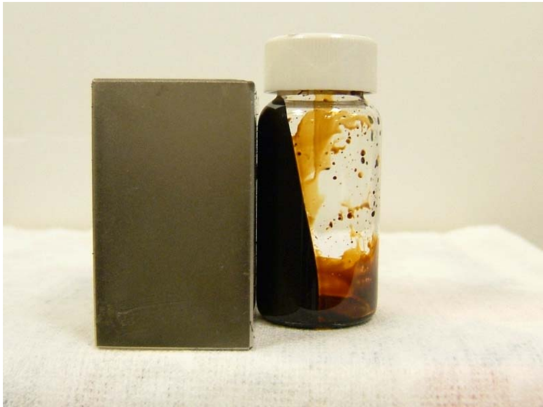
Figure 3.8 The magnetic effects on the \text{Fe}_3\text{O}_4 nanofluid
