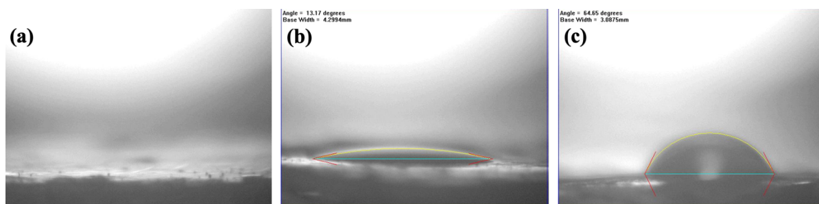
Figure 4-36. Contact angles measurements of (a) Cu/ZnO/Al 2 O 3 ; (b) 20CZALa/hBN; (c) h-BN
