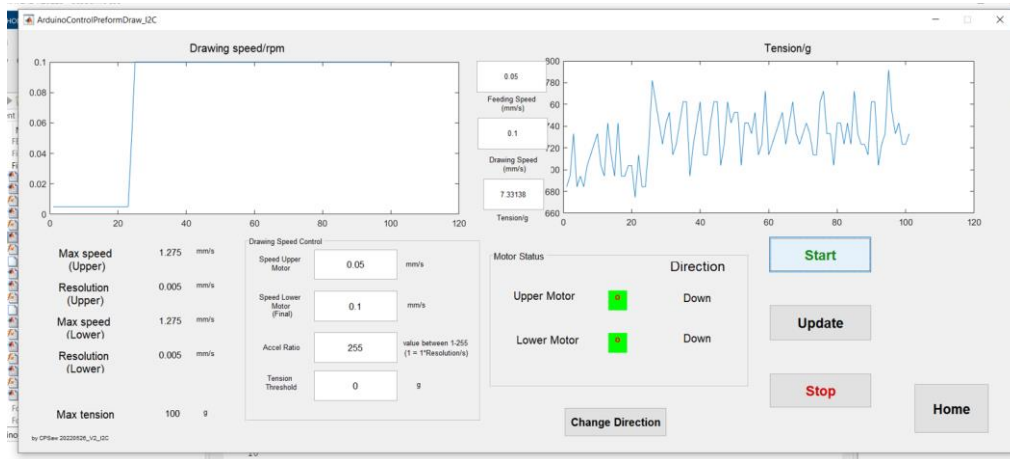
Fig. 2-27 MATLAB GUI for controlling the two stage preform drawing system
