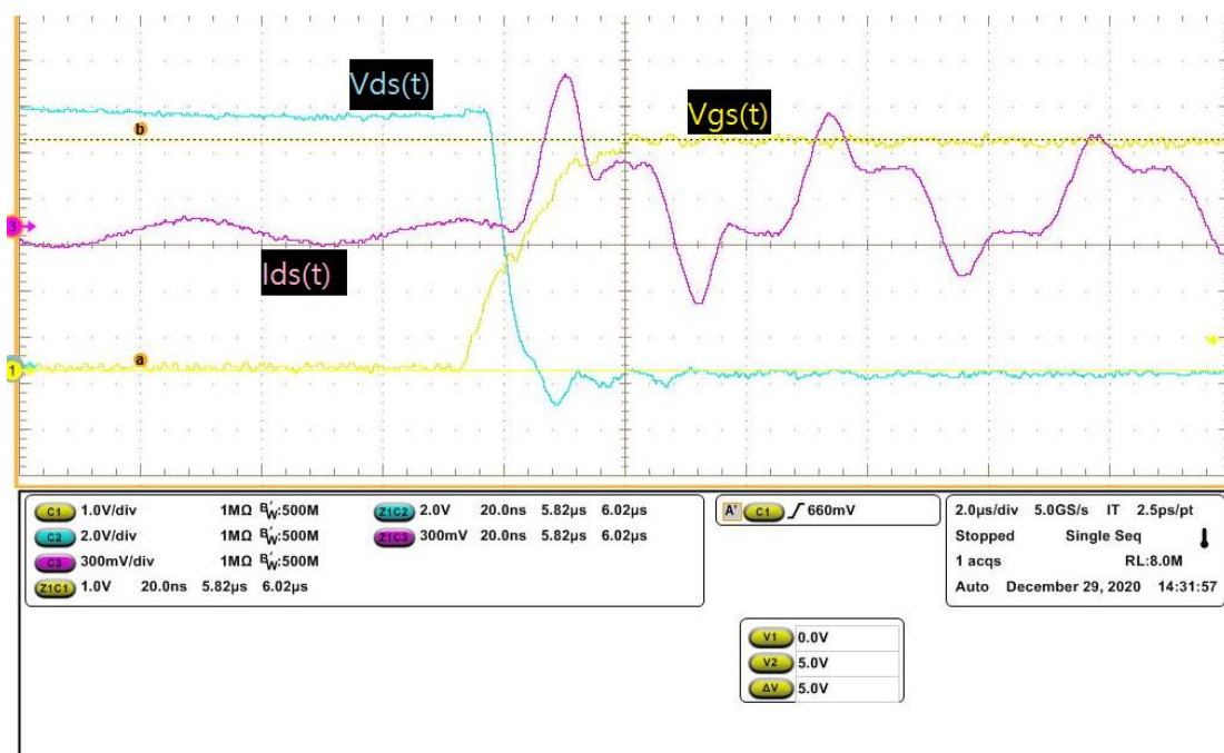
Fig. 5.13 Waveforms of board F when 10V/2A is applied
