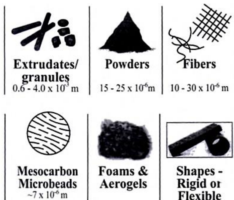
Figure 2-4 forms and properties of activated carbon (Derbyshire et al., 2001)
