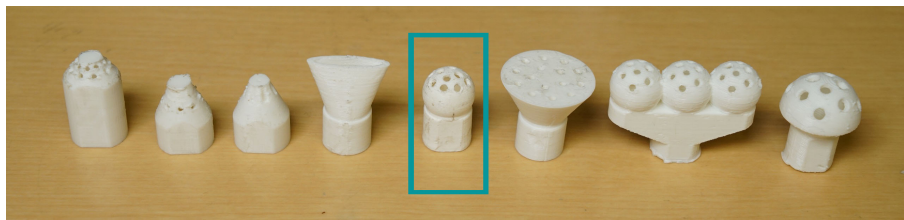
Figure 4.2: A variety of nozzle designs we explored and evaluated to maximize airflow coverage and uniformity.
