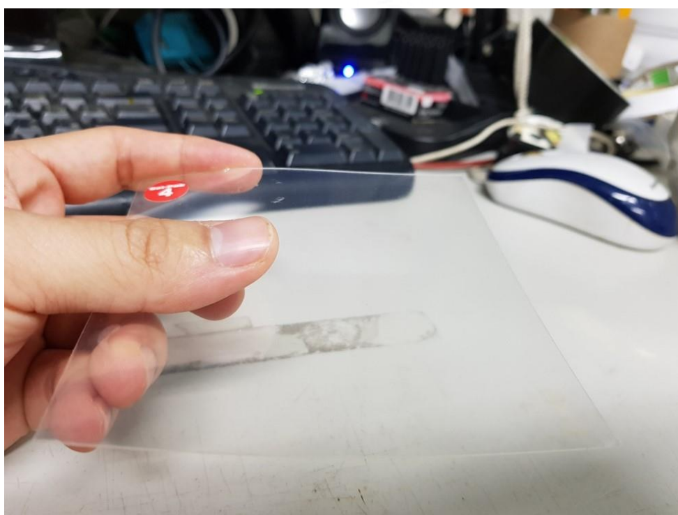
Fig. 2.3 The PDMS stamp used in this research.
