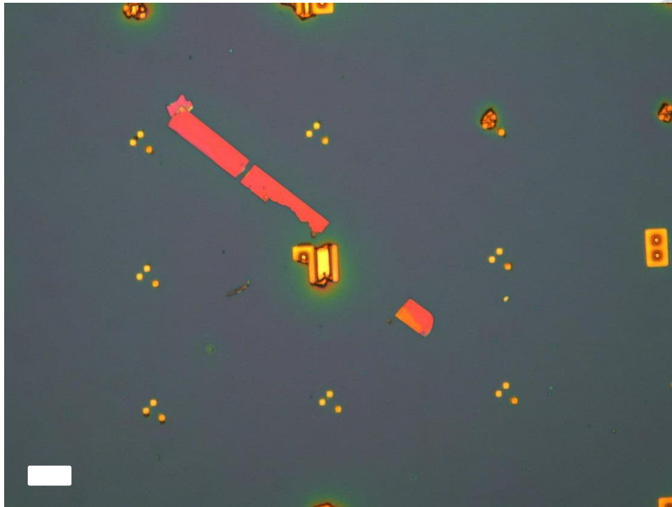
Fig. 2.4 Exfoliated rectangular BP on 300nm SiO 2 /Si substrate under optical microscopy. Scale bar is 20um.
