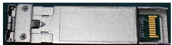
Figure III.20: Placement of a SFP cover into a SFP cage.
