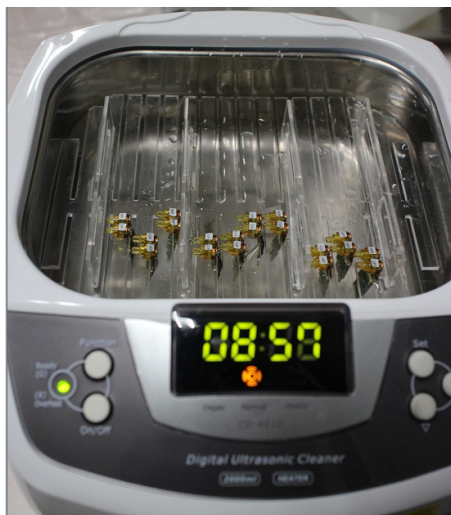
Figure III.8: Ultrasonic cleaner for solder paste cleaning.
