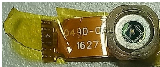
Figure II.19: A TOSA without focusing lens.
