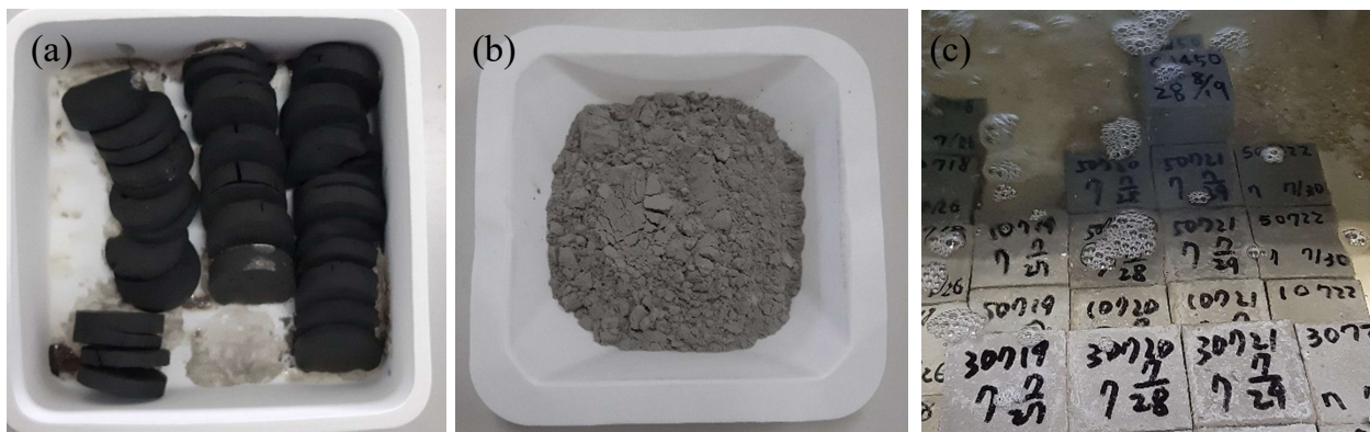
Figure 5. Pictures of (a) the clinker after sintering, (b) cement powder, and (c) cement mortar in cured period.
