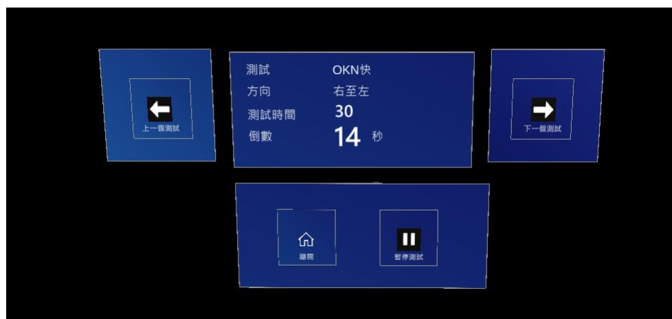
Figure 3.1: The screenshot (captured in the editor) of application records the eye movement in HoloLens2™. The application is built with Unity3D (Unity®), using the Mixed Reality Toolkit (MRTK-Unity) developed by Microsoft®.
