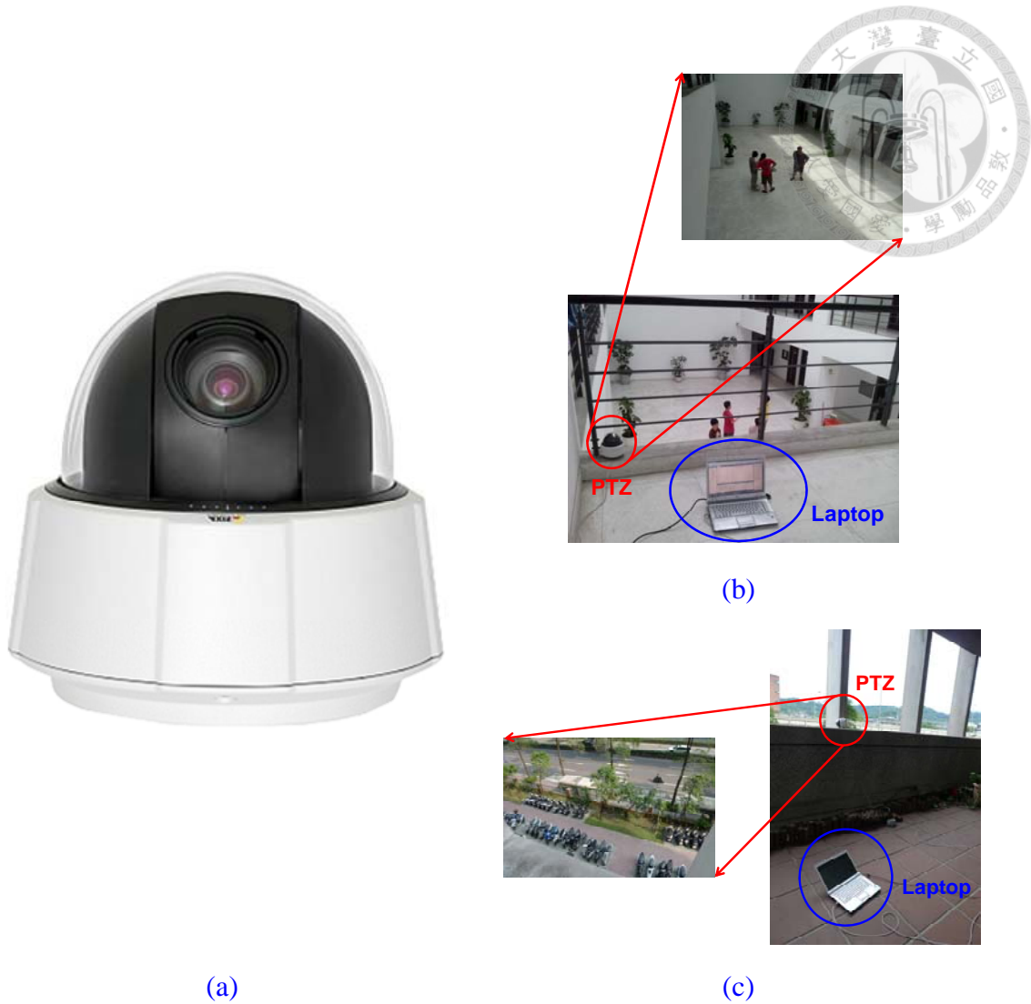
Figure 3.4. (a) AXIS P5512 PTZ camera used in the dissertation. (b) Indoor experimental scene at MD building in NTU. (c) Outdoor experimental scene in NTU.
