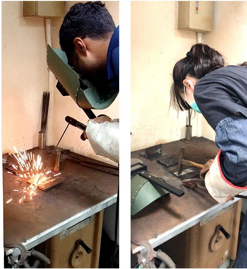
Fig. 3.16 (a) Real welding task and (b) Chip removal from the welded joint
