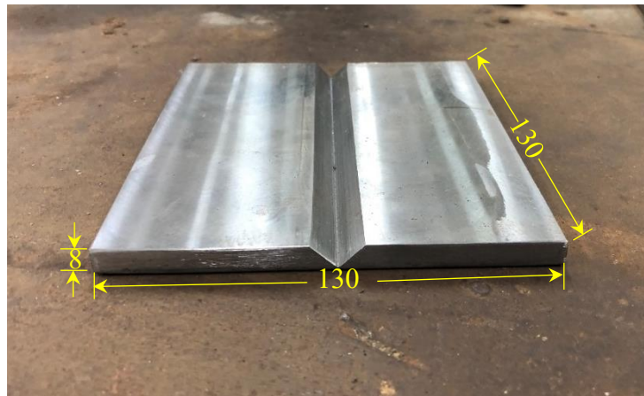
(a) Workpiece for butt joint
