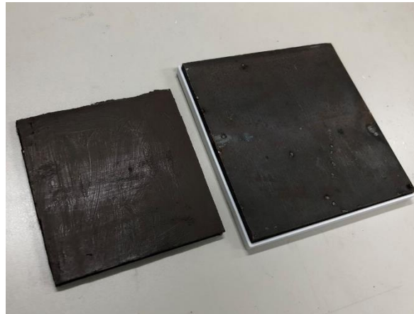
(b) Real dummy plate (left) and workpiece in a fixture (right).
