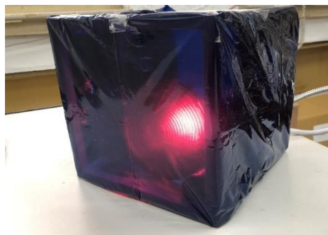
Fig. 3.3. Infrared heat lamp inside a box made of translucent plastic foil.
