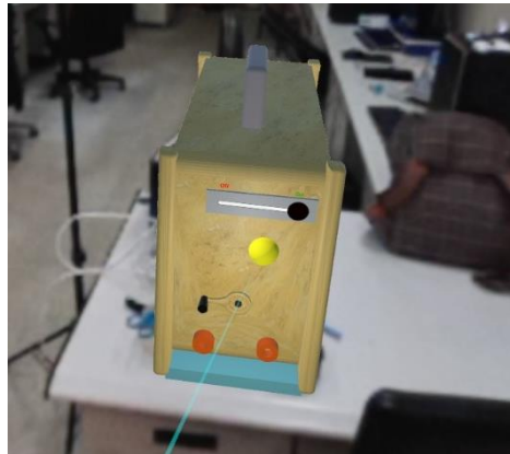
Fig. 3.9. Switching on the welding power source.
