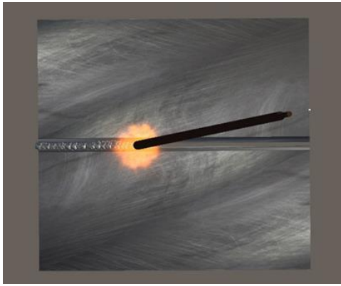
(a) Pulling technique (top view)
