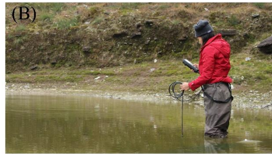
Plate 2 Environmental parameters recorded by (A) the Turner Designs C3™ submersible fluorometer and the Greenspan DO100 dissolved oxygen sensor on the buoy which deployed above the deepest spot of lakes and by (B) the YSI Proplus multimeter
