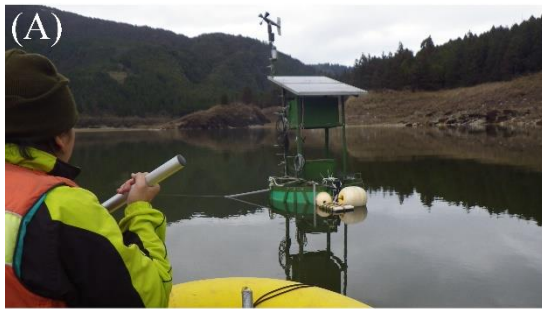
Plate 2 Environmental parameters recorded by (A) the Turner Designs C3™ submersible fluorometer and the Greenspan DO100 dissolved oxygen sensor on the buoy which deployed above the deepest spot of lakes and by (B) the YSI Proplus multimeter
