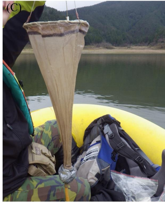
Plate 4 (A-B) Sampling the benthic macroinvertebrates with (A) direct picking from the bottom substrate and (B) retrieving macroinvertebrate individuals from sets of colonization tiles in meshed bags pre-deployed 3 - 6 weeks prior to collection. (C) Zooplankton sample was collected by hauling a vertical zooplankton sampling net from lake bottom to surface
