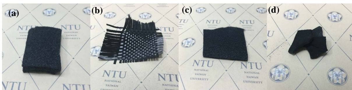
Fig. 2-8. Electrode materials used in MFCs: (a) carbon felt, (b) carbon fiber, (c) carbon cloth and (d) graphite.
