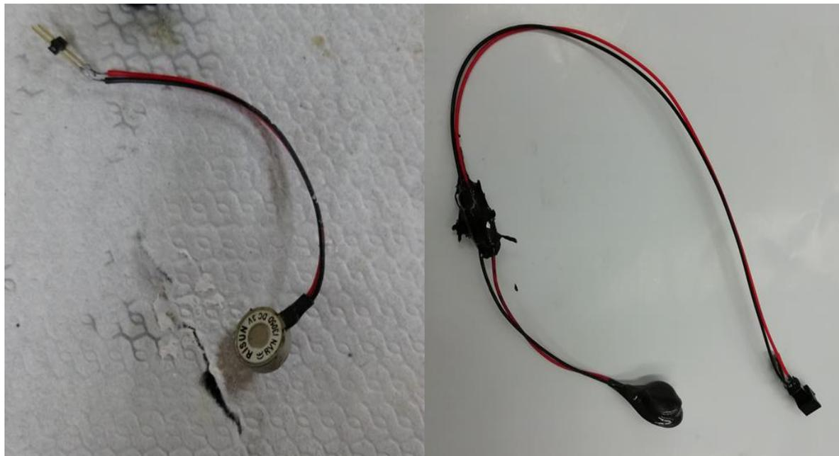
Figure S4-2. Photo diagrams for commercial motors (RISUN PVN 1305D 3V) before (left) and after (right) coated with layers of Hg-free epoxy resin and plastic steels.
