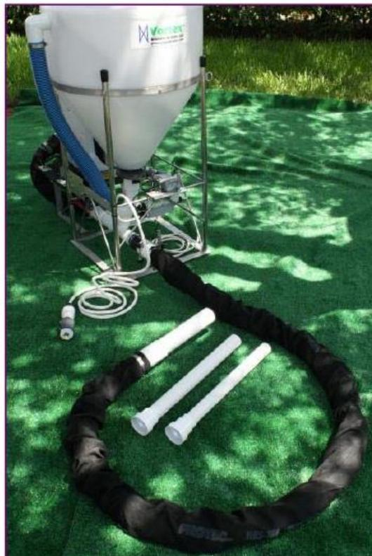
Figure 2-2. Menzie et al. [62] performed a spray thin layer capping using self-made equipment (Vortex TR Aquatic system).
