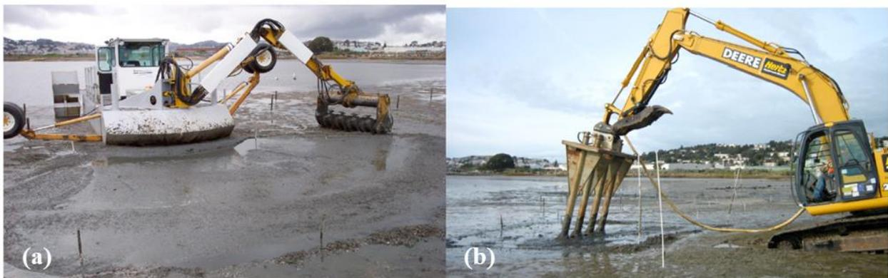
Figure 2-1. Cho et al. [8] performed mechanical mixing amendment with (a) a rotary cultivator (Aquatic Environments, Inc.,) and (b) an injection system (Compass Environmental, Inc., GA).
