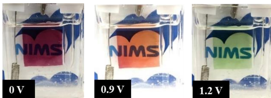
Fig. 3-3 Images of PolyRuFe at 1.2 V (bleaching state), 0.9 V and 0 V (coloring state) in three electrode system (vs. Ag/Ag + ).
