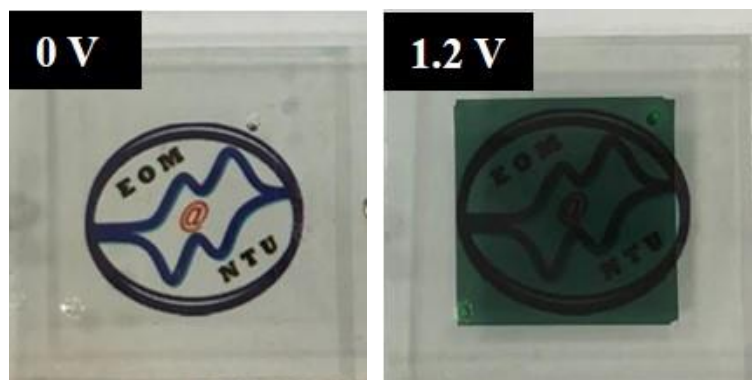
Fig. 4-21 Images of NMP-IL/PV ECD at coloring state (1.2 V) and bleaching state (0V).
