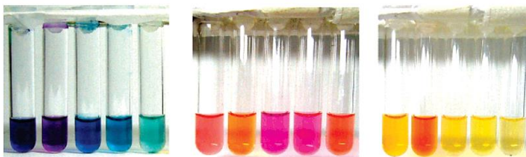
Fig. 1-2 Colors of \text{Fe}^{2+} , \text{Ru}^{2+} , \text{Co}^{2+} based metallo-supramolecular polymers and with various ligands L1 to L5, respectively 25 .
