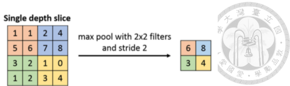
Fig. 2. 8 The example of how the max-pooling with 2 \times 2 mask and the stride 2.
