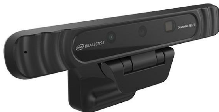
Figure 4-12. Depth sensor. This figure shows the depth sensor used in the testing, which is Intel Realsense.
