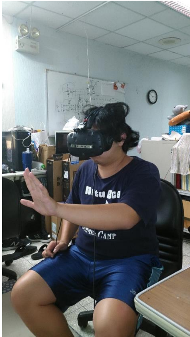
Figure 1-1 The device we have used in our experiment, which is a HMD (HTC VIVE) attached with a depth sensor (Intel RealSense F200). We take the depth image by the depth sensor and reconstruct the hand model in the VR world.
