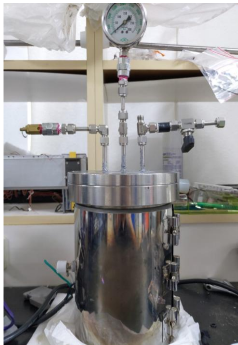
Figure 3- 10. The steam generator.
