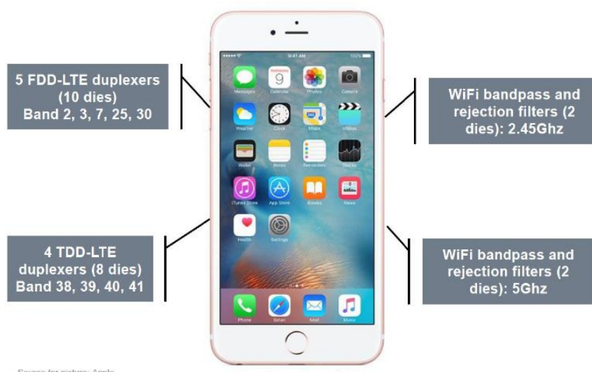
Fig. 2.5. Example BAW filters used in iPhone 6(EPFL online course MEMSx).
