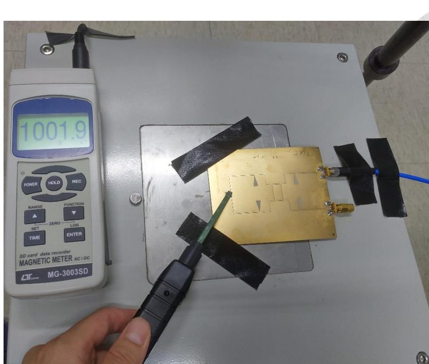
Fig. 4.15. The adjustable permanent magnet is meant to provide necessary out-of-plane magnetic field to saturate the device. One tesla is measured near the surface of the chip using a DC magnetic meter MG-3003SD.
