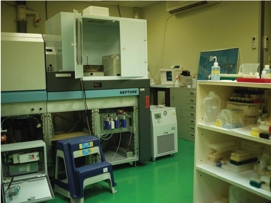
Fig. 2-5 MC-ICP-MS with SEM protocols, Thermo-Fisher, Neptune, used for U-Th isotopic measurement.
