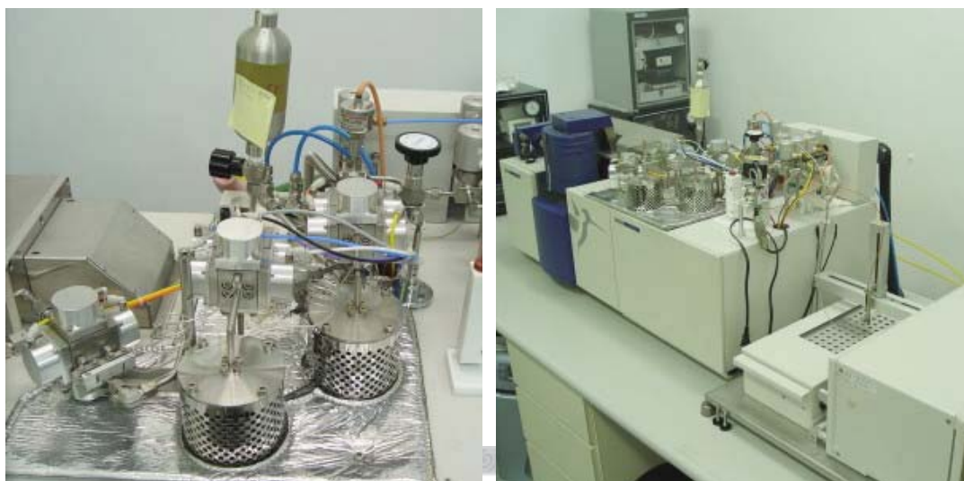
Fig. 2-6 Micromass IsoPrime IRMS used for the oxygen and carbon isotope analyses.
