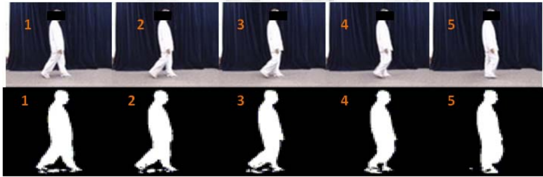
Figure 3.3 An example of gait image processing: top: original color image frames, bottom: binary silhouette frames.
