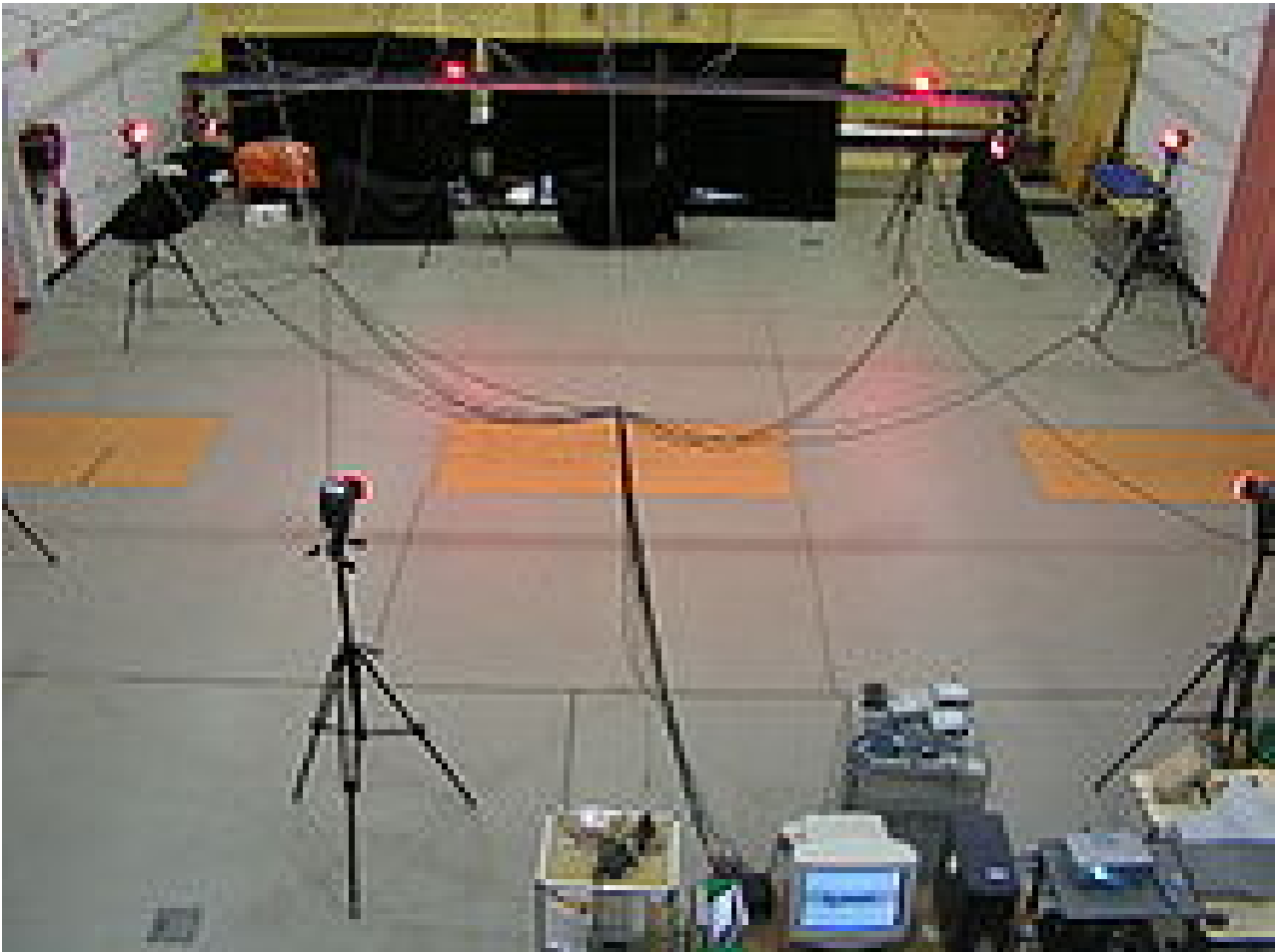
Figure 1.3 A gait laboratory with lighting condition, passive infrared cameras, and embedded force platforms
