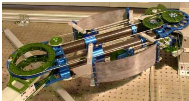
Figure 3-6 An Actuator with Mechanically Adjustable Series Compliance [52]
