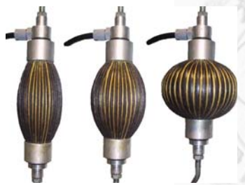
(a) Pleated pneumatic artificial muscle [74]
