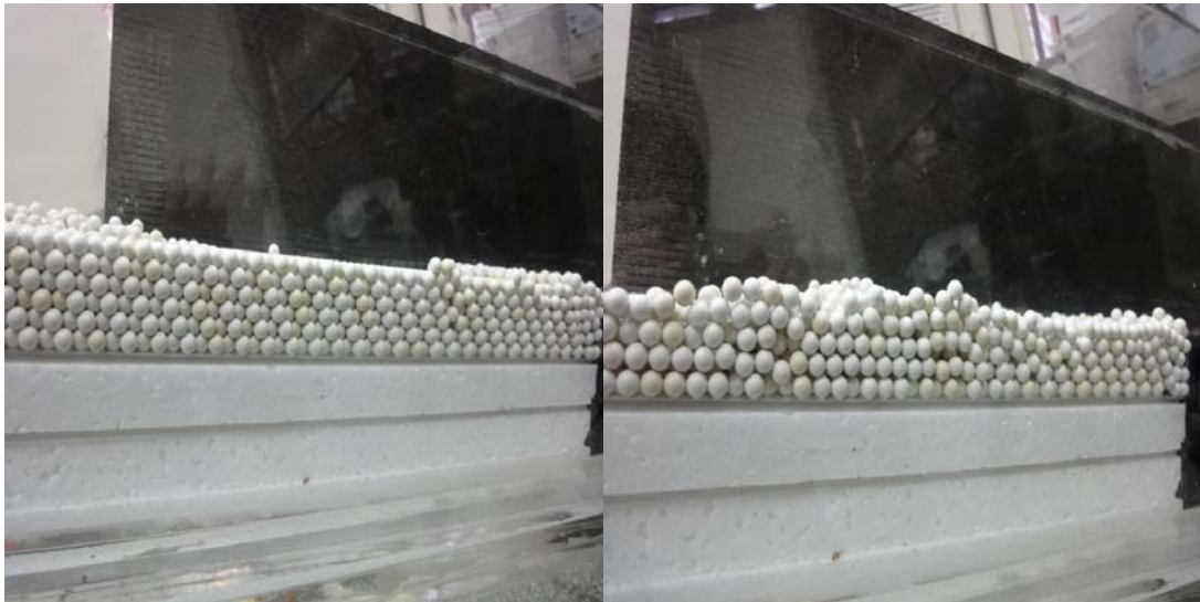
Figure 5.3 Packing formation for the spheres arrested in front of the impact load cell for chute of 2.4 cm depth and 20° inclination: (a) close orderly packing and (b) loose and random packing.
