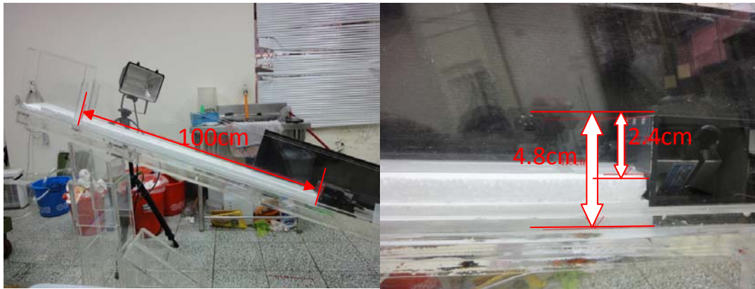
Figure 5.1 Experimental facility: (a) the chute and where the load cell module was installed; (b) flow depth h from the load cell top surface to the base.
