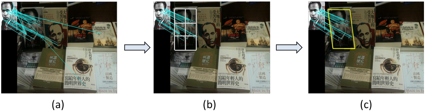
Figure 4.3: The steps of getting affine model: (a) original feature matching pairs after object recognition system, (b) counting a grid-based feature density matrix after removing incorrect feature matching pairs, (c) calculate affine model by three random features which are from three different high density grids.
