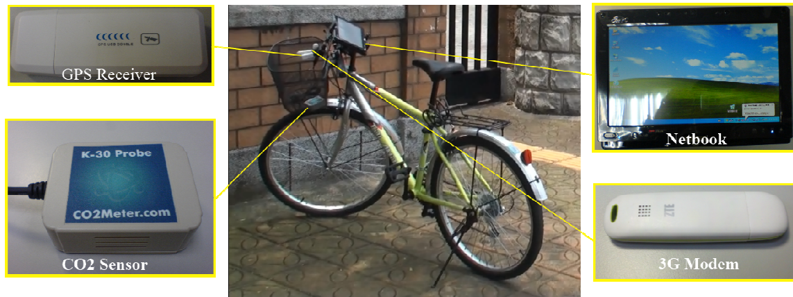
Figure 5.3: A bicycle equipped with a netbook, a GPS receiver, a CO 2 sensor, and a 3G modem
