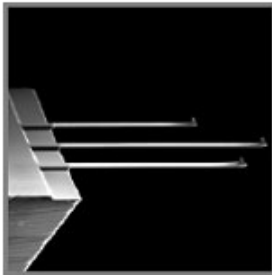
SEM image of 3 cantilevers (A, B, C) on chip of the CSC38 series.
