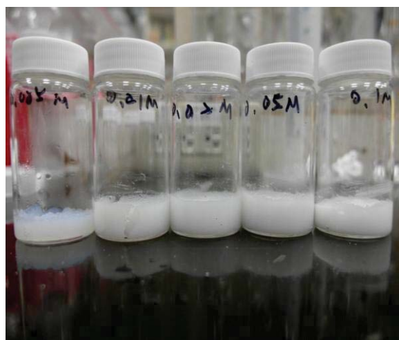
Figure A.1 The ZrO_2 gels with different concentration of precursor dried to certain state. ( ZrO_2 (0.01M) just cracked and others were not far from cracking)
