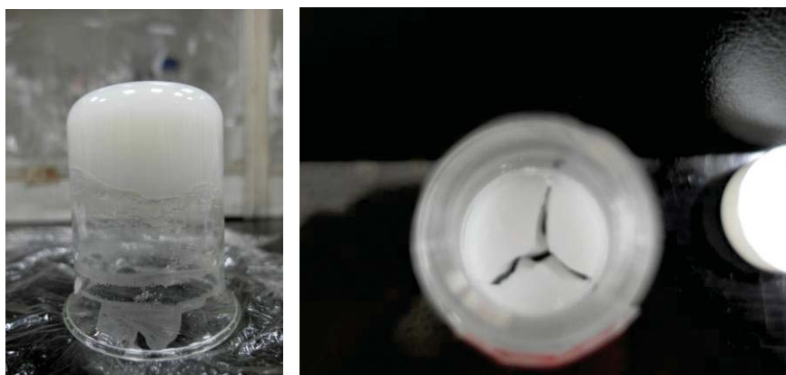
Figure A.3 (left) The viscous gel property of ZrO_2(0.01M) -Dry 23hr (right) The crack image of ZrO_2(0.01M) -Dry 23hr.
