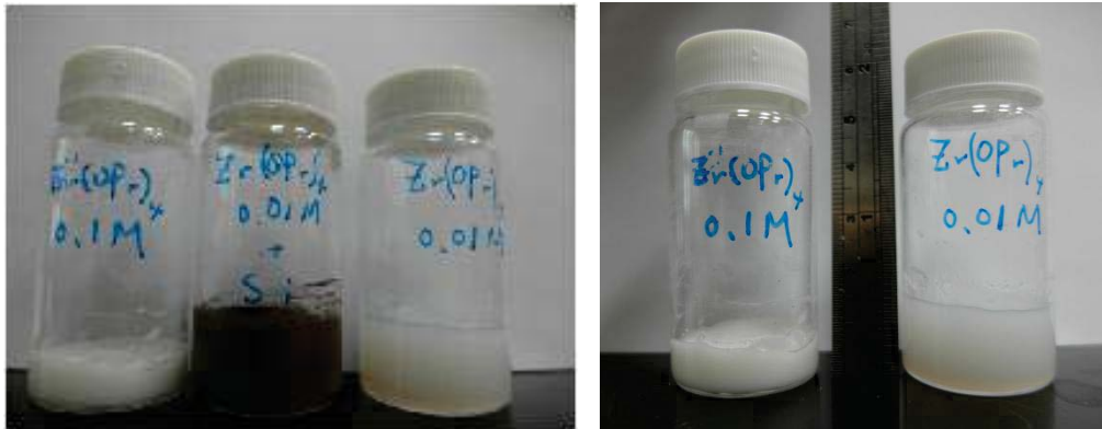
Figure A.6 (Left) Z(0.1), Z(0.01)S(40), and Z(0.01) gel from left to right. (Right) the huge difference of left volume when crack just formed of Z(0.1) and Z(0.01) gel samples.
