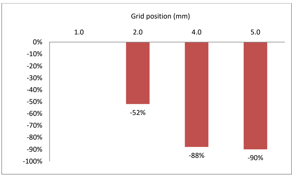
Fig. 31: 4.0S*9.0 mm Astra Tech implant: (a) the MSV of micro-strain gauges at four different heights. The error bar is the positive and negative standard deviation of each group of data. The R^2 of logarithmic regression line is 0.967; (b) the MSV decreasing rate of the three strain gauges below 1.0 mm. The largest value occurs at the 2.0 mm.
