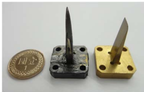
Figure 5.1 Copper wedge-shaped base (right) and wave absorber with a lossy conducting layer (middle).
