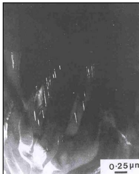
Figure 2-11 The observed fibrous carbides in pearlitic ferrite, a dark-field image [5]
