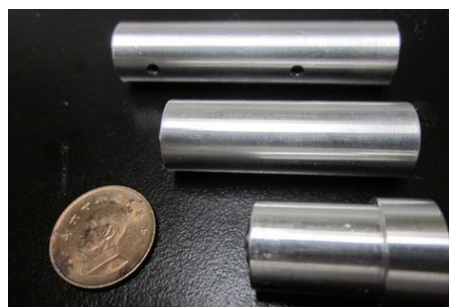
Fig 4.10 Replaceable tube lens pairs, the magnification ratio is 1:1.5, 1:3, and 1:1 (top to bottom).
