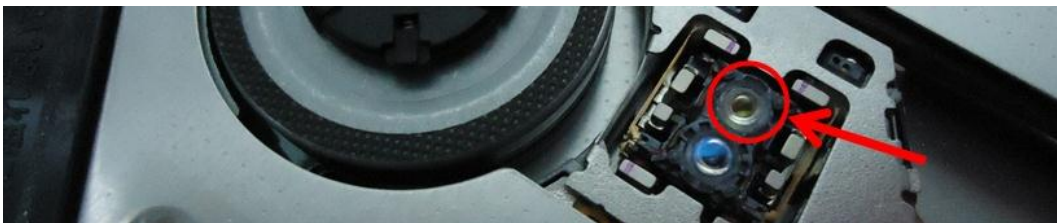
Fig 4.4 Dual lens pair in an optical disk drive, where the marked on is the BD lens and another one is the DVD lens. A simple way to distinguish these two lenses is to observe their reflective light. The surface coating for the BD lens is highly transmitted for blue light, so it will reflect yellow light; whereas the DVD lens is highly transmitted for red light, thus it will reflect blue light.
