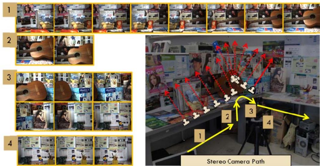
Figure 6.6: Camera path and corresponding image captured from right CCD
