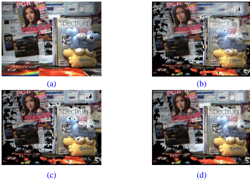
Figure 6.20: Illustration of the concept of using PSNR as similarity index to compare the 3D reconstruction quality in the color space viewpoint.
