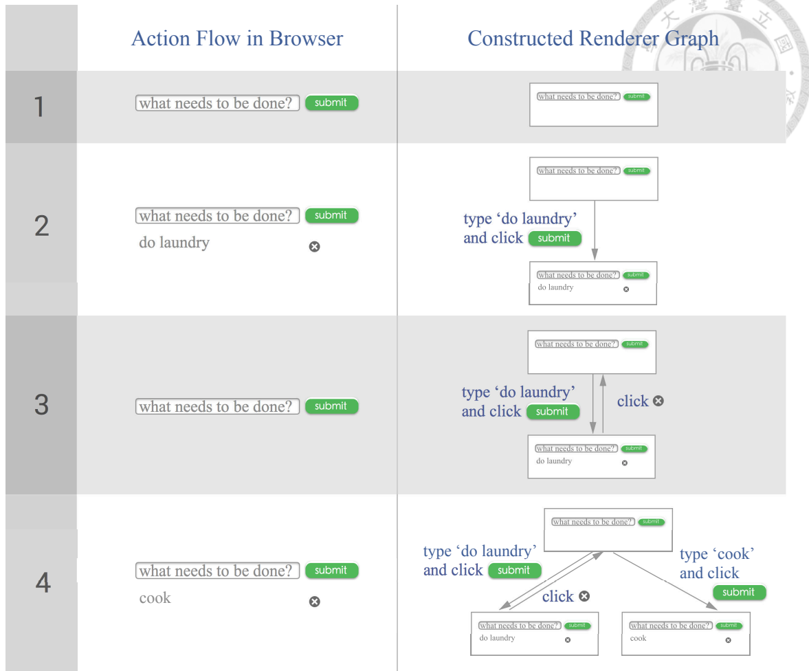
Figure 7.2: Constructing the Renderer Graph as the developer manipulates the To-Do list web application. Each step that updates the user interface would create a new renderer in the renderer graph. The developer performs the following steps, resulting in the renderer graph on the right: Step (1) the browser reloads and displays an empty to-do list. Step (2) developer submits a new item. Step (3) the new item is deleted by the developer. Step (4) developer submits another new item.
